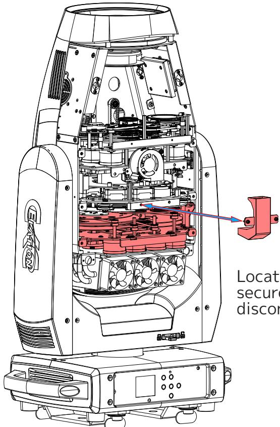
Locate the Gobo Module, remove the screws that secure it to the internal housing frame, and unplug/ disconnect wire harness.
