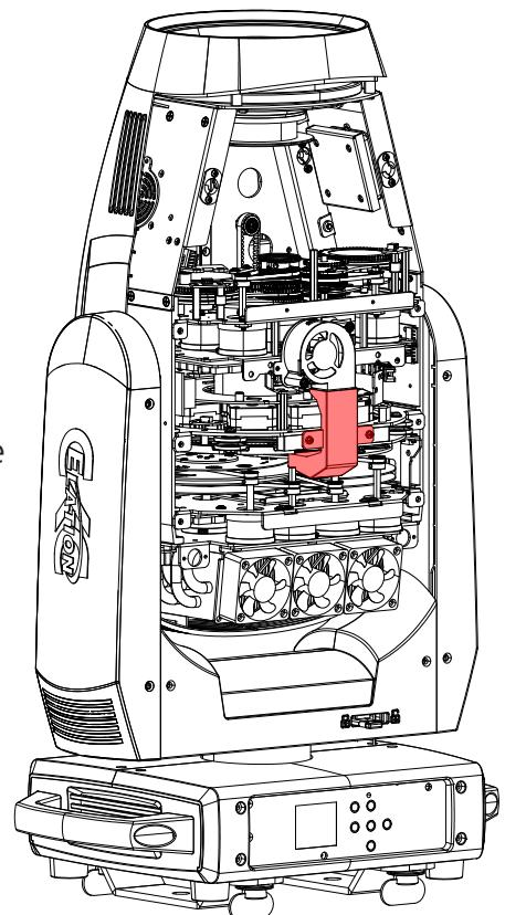
Locate the Fan Ducting, remove the 2x screws that secure it to the internal housing frame..
