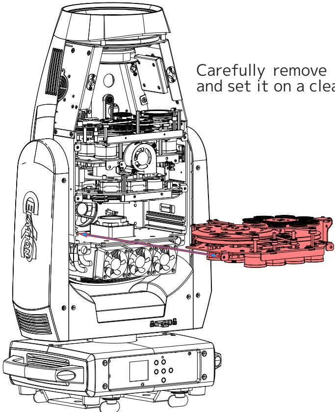
Carefully remove the Gobo Module and set it on a clean surface.
