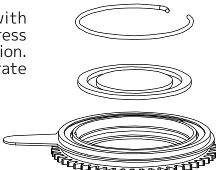
**Note:** To ensure proper Gobo orientation on the Rotating Gobo Wheel, align the Alignment Indices before installing the Retention Spring.
