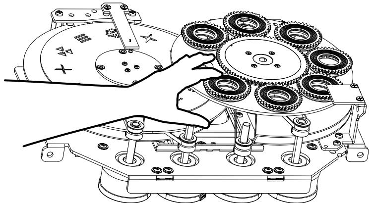
Locate the specific Rotating Gobo to replace. Carefully grip the Gobo using your thumb and index finger, gently lift it slightly, and then pull it out and away until it fully clears the Gobo Wheel.
