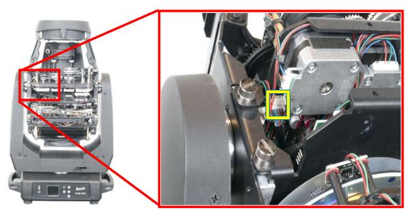
3. <u>Optional. This step may be performed to help improve access to the gobo wheel</u> <u>module.</u> On the prism module, find the 4-pin connector (denoted by the yellow box, above right) in the that is located behind the left-most electric motor, just beside the thumb screw on the left hand side of the prism module. Disconnect this connector.
