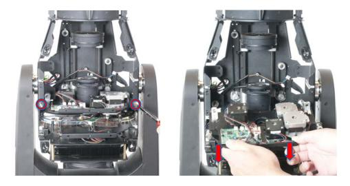
6. Loosen the thumb screws for the gobo wheel module, and carefully slide the gobo wheel module out of its mounting slots. Place the module on a flat, stable surface in a **DUST-FREE**, **INDOOR** location.
