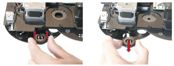
7. Locate the rotating gobo that will be replaced. Grip the edges of the geared gobo holder and gently lift (pictured at left) until the gobo holder clears the surface of the gobo wheel. Then pull the gobo holder out and away (pictured at right).
