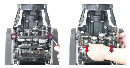
4. <u>Optional. This step may be performed to help improve access to the gobo wheel</u> <u>module.</u> Loosen the thumb screws for the prism module, and carefully slide the prism module out of its mounting slots. Set the prism module aside for later reinstallation.
