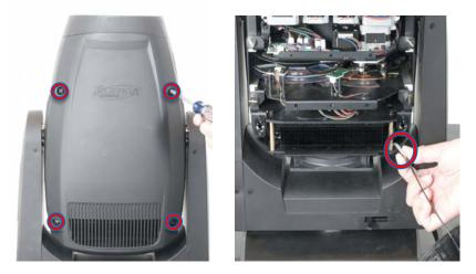
2. Use a Phillips head screwdriver to loosen the four (4) fasteners on each of the covers. **Please note that these fasteners are of the twist-lock variety, and do not come free of the covers.** Remove the safety cable clips securing each cover to the fixture.
