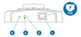
RJ45. Powered over Ethernet
