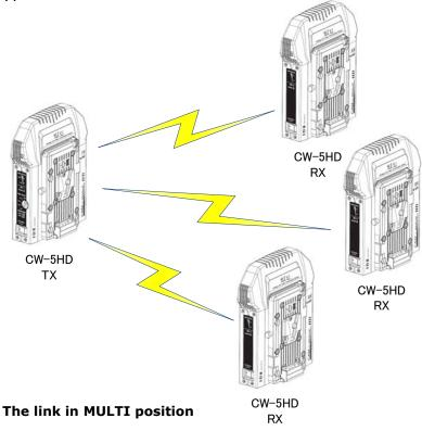
There is no limit on the number of receiving CW-5HD RX in MULTICAST mode as long as they are within reach of the transmitted signal and existing environmental conditions are taken into regard.
