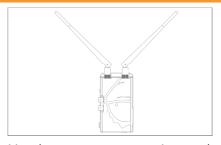
Position the antennas on transmitter as shown in the illustration. This ensures the best possible RF performance.
